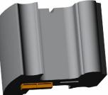
Key to be inserted in base of block - the degree of setback placed towards the front of the block.
