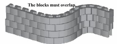
Curves cause the lead and lag of the block over the one below it to change. It is caused by the change in radius of each curve over the one below as the wall goes up and back. A curve in the first course that is too tight cannot be continued up through the wall. The more exotic the wall, the more likely masonry cuts will have to be made.
